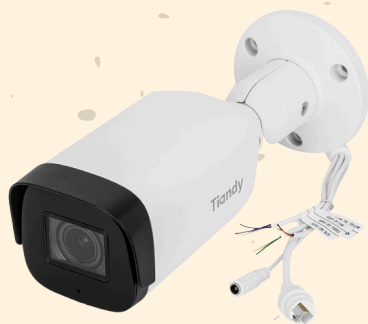
TC-C38US SPEC:LK/I8/A/E/Y/M/S/H/ 2.7-13.5MM/V4.0 8 MPX / IR 80M
