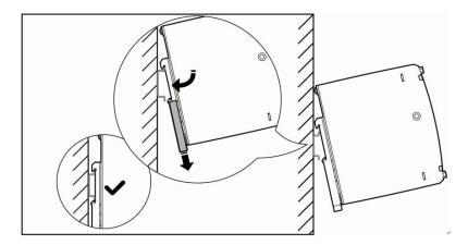
(2) Connect the power module to the switch, as shown in the following figure.
